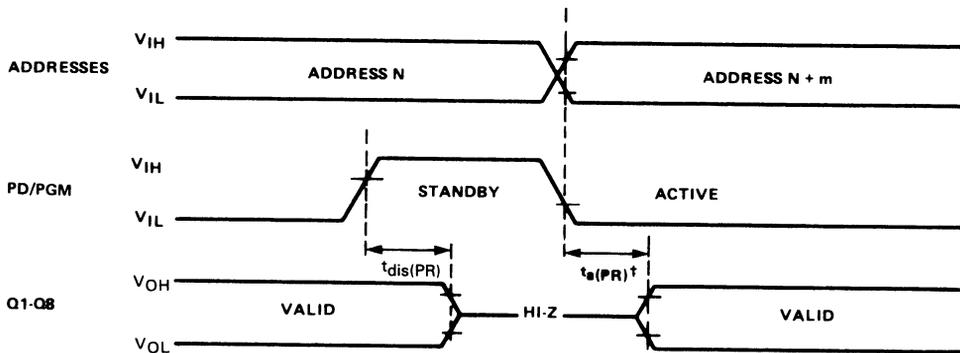
NOTE:  $\overline{CS}$  must be in low state during Active Mode, "Don't Care" otherwise.
